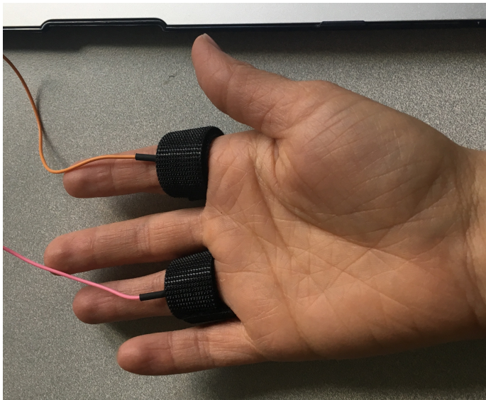
Figure 4. Placement of GSR electrodes.
